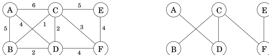
Figure 5.1 The minimum spanning tree found by Kruskal's algorithm.
